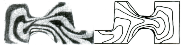
Fig. 6. Metal flow of forged gear blank obtained from plasticine simulation (left side) and from CAE analysis (right side).
