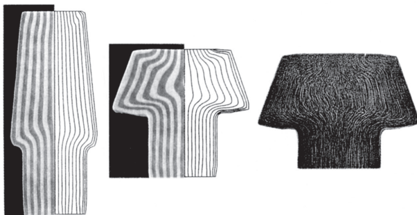
Fig.14. Comparison of metal flow in differential gear blank, plasticine experiment, and FE analysis .
