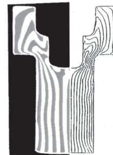
Fig. 15. Comparison of plasticine experiment (left side) and finite element analysis (right side) on metal flow. (sun gear 4th process shown in Fig. 6, lubricant:CaCO 3 , friction:sticking)
