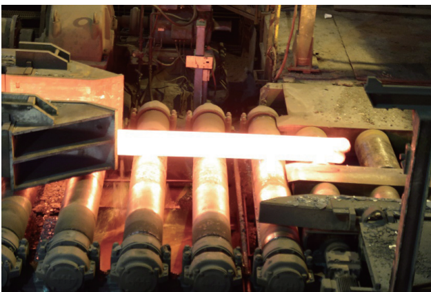
Fig.6 Hot rolling test
