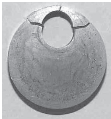
Fig.15 Cracks occurred in SK4 steel disk with an eccentric hole by water quenching 46) .
