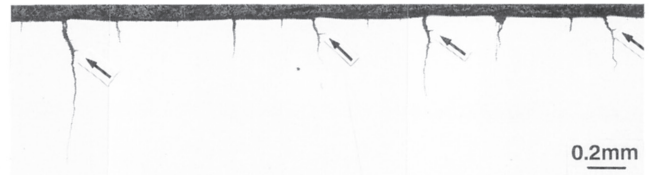
Fig.9 Cross sectional view of heat checking with branched cracks.
