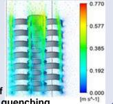
Simulation example of oil flow in furnace oil quenching
