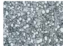
SPC5 焼入れ: 1150°C × 8min O.Q. Quenching 焼戻し: 500°C × 1h A.C. × 2 Tempering
